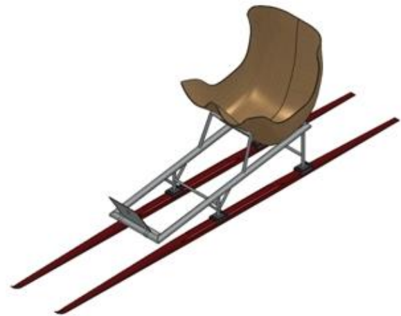
Fig. 6.7. Computer model of the custom Sit Ski.
